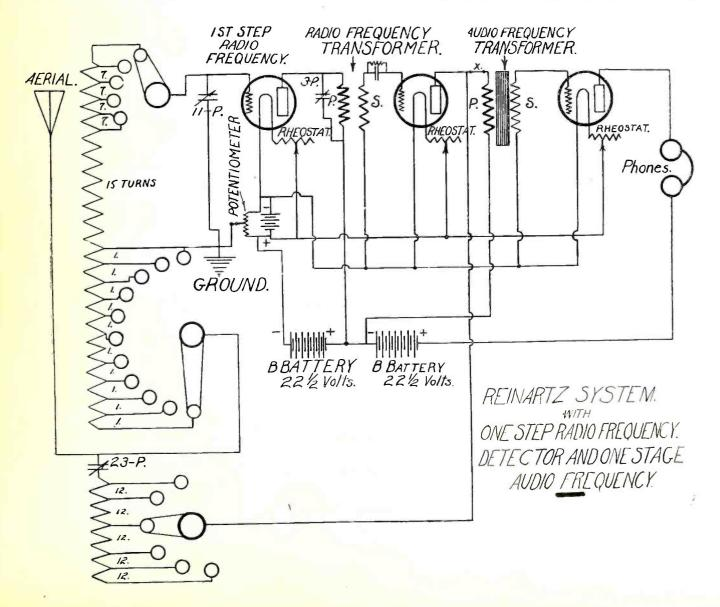
radio frequency. They are then carried to the detector tube, where they are rectified and brought down to audio frequency. From this it will be seen that radio frequency amplification will really magnify oscillations received upon the aerial and pass them to the detector tube for rectification.
